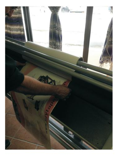
Pull the print and the laminate through, without removing the laminate backing, to make sure everything is tracking properly. (For smaller prints, it's usually easiest to pull the media with your hands, but for larger ones, you might want to use the crank.) Then, if everything is OK...
