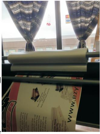
Step 12 A quick visual to check that the backing sheet is tracking with the print.
