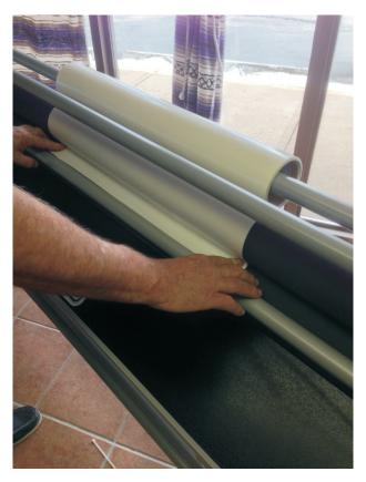
Roll the laminate through. I only use my hand on the roller -I do not use the crank. Then back roll and unfold the crease, leaving just enough vinyl exposed to touch the cut-off rail. Now, back roll the laminate on top just enough to tension up the slack.
