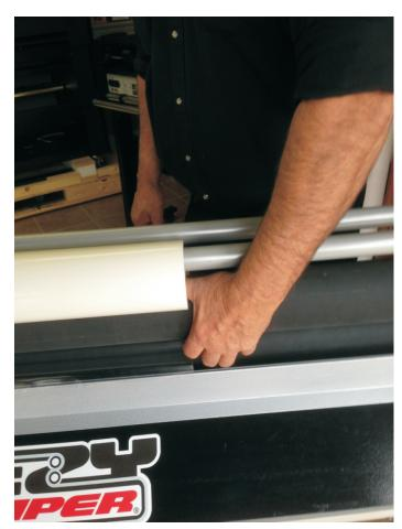
Step 9 Just a reverse view of me holding the top roller with my thumb hooked to the roll of laminate while I pull the backing sheet over the top of the roll of laminate
