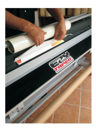
Peel the backing paper off the laminate and tuck under.
