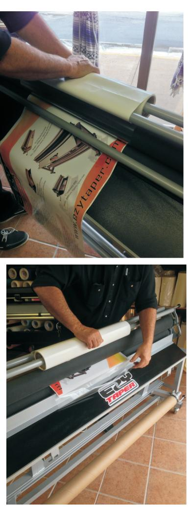
Stop with the backing sheet about half the way around the top roller. At this point you want to make sure that the backing sheet is tracking true to the edges of the laminate. At this time adjustments can be made for trueness without harming the print
